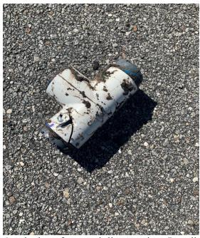
Cracked tee from mainline repair at Paradiso and Waterset Blvd.
